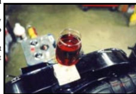
Not a ripple at 3000 RPM
